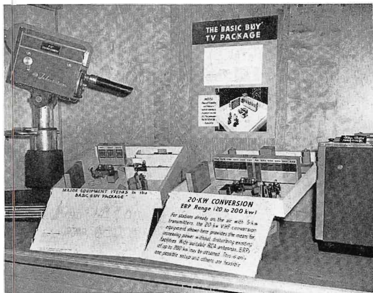
Display of the RCA "Basic Buy" for television broadcasters and 20-kw conversion equipment which enables 5-KW stations to obtain up to 200 kw (ERP).
