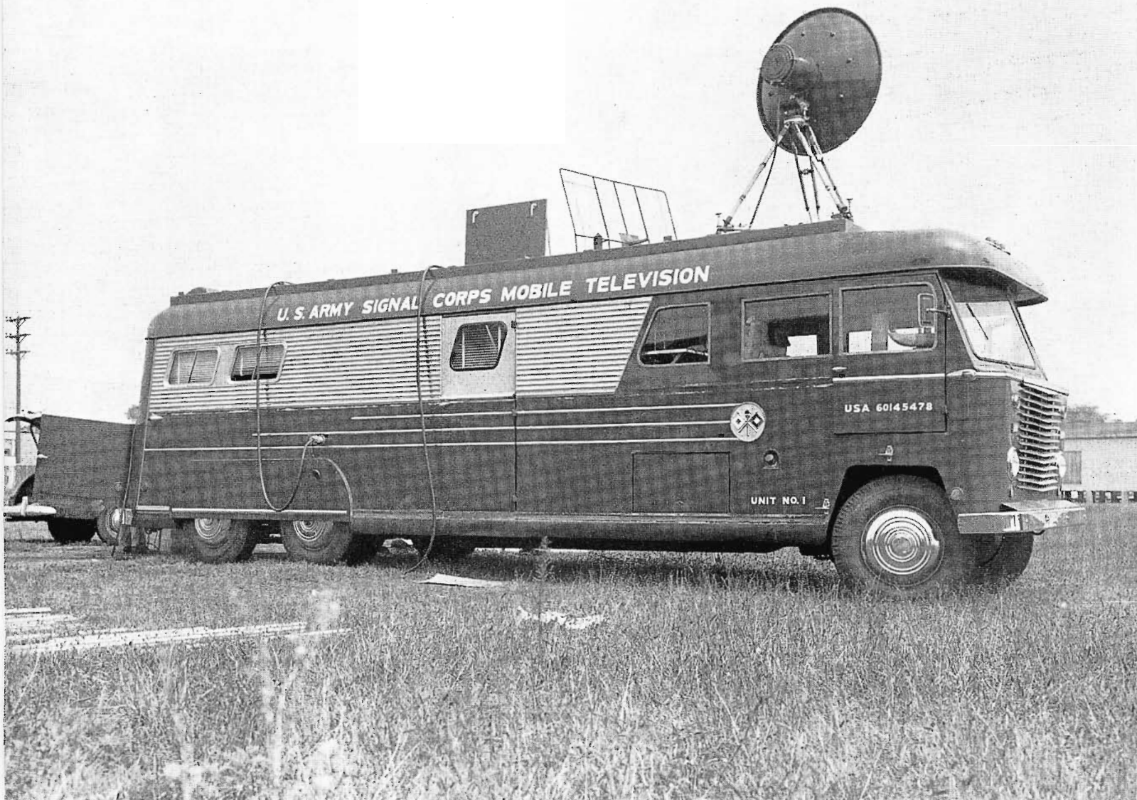
TRANSMITTING unit above contains TV cameras and microwave transmitting equipment. A monitor-control position is built into the rear of the vehicle.
